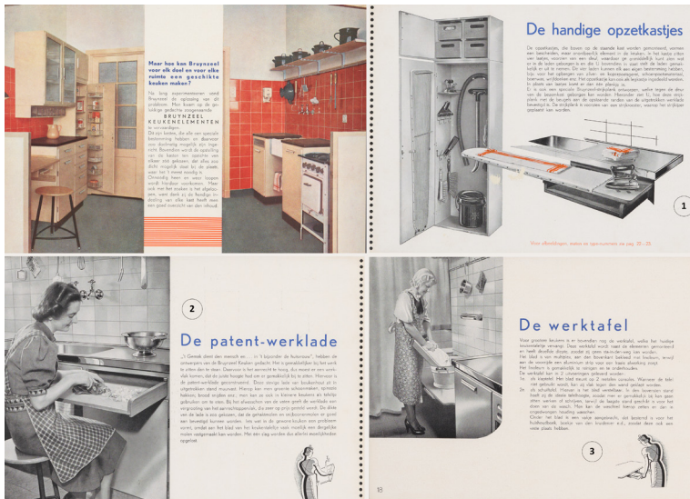
Figure 8 Pages from a Bruynzeel folder explaining various smaller handy tools such as: 1) handy opzetkastjes (elements to attach) for ironing; 2) extendable werklade (work drawer); 3) the removable werktafel (work table) (Image from Nieuwe Instituut/MEIJ, d7; annotations by authors)
