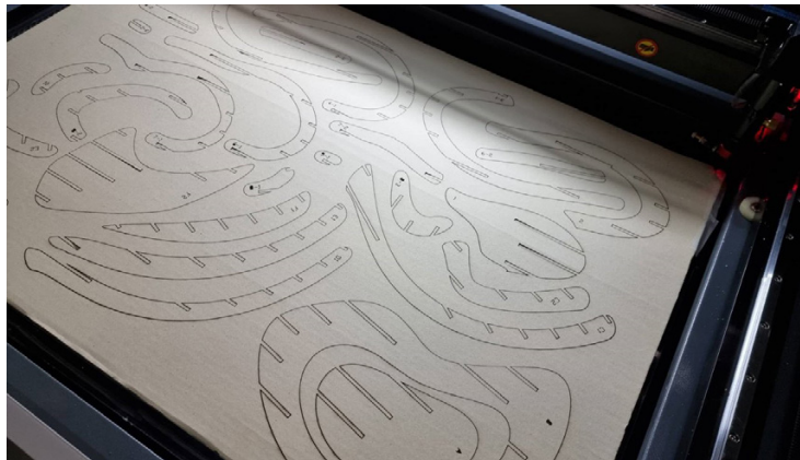
Figure 11 Cardboard material cut by a laser cutter for further assembly (Photograph by authors)
