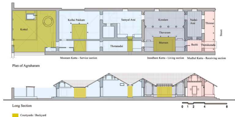
Figure 4 Plan and section of agraharam showing three main sections (Image by Himani Shingala and students of IIDEA, Indus University)
